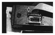
14. Attach black plug of replacement ribbon cable to air condition control unit
