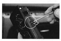
7. Unclip and remove air condition control unit
