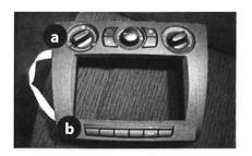
15. Attach air condition control unit(a) and switch bar (b) toreplacement facia plate
