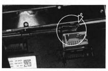
6 Unclip and remove switch panel below air condition control unit
