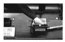
5. Remove plug attached to ribbon cable
