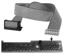
13. Attach white plug of replacement ribbon cable to PCB
