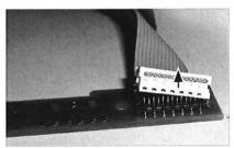
12. Remove plug attached to ribbon cable from PCB
