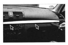
2. Unclip middle panel and remove it carefully
