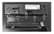
11. Remove 5 screws from switch panel ( see arrows)
