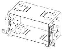
16. Set metal frame into dashboard and fix it with screws
