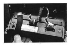
4. Pull out air condition control unit carefully
