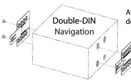
Attach mounting brackets to double DIN navigation
